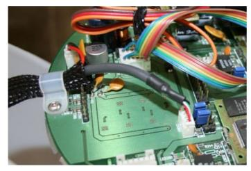
Plug in the USB (4 pin) and power (2 pin) plugs of the new cable. Check that the plugs are inserted the correct way round.
