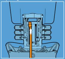
5 Connect the 24v power cord located under the rear cover
