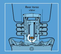
4 Connect the multicoloured connector and the network cable
