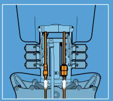
3 Connect the airline firmly pushing into the black fitting
